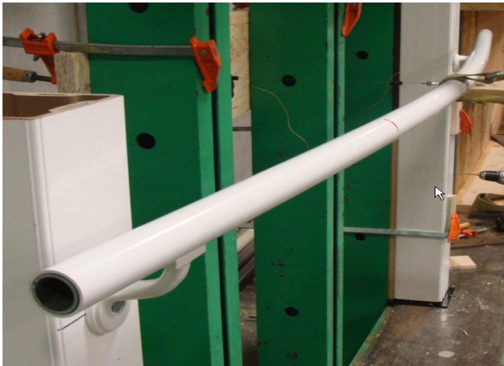
PHOTO 4: 200 lbf Load Applied – Horizontal Midspan
