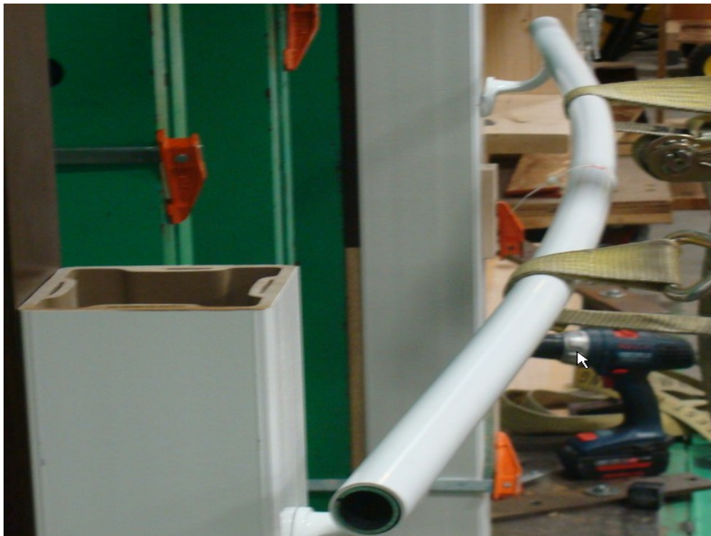
PHOTO 8: 50 plf Load Applied – Horizontal (photo taken at 300 lbf)
